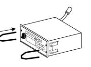
In order for the radio to be removed, clips attached to the side of the radio must be moved inward so the radio can slide out of the dash. Insert the keys and push each key out, away from the radio. The ends of the keys will press into the clips. While pushing the keys outward, pull and the radio should slide forward out of the dash.
