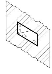
New radios 'DIN' cage slid into the 'DIN' opening of the dash with its tabs bent securing the cage to the dash.
