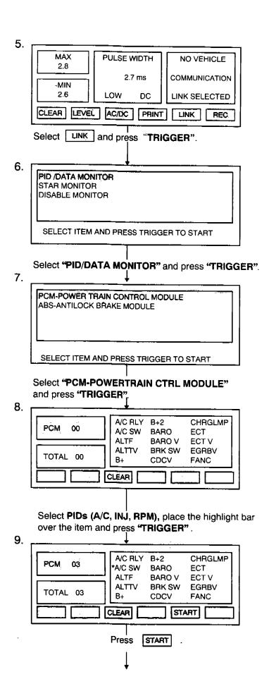
The screen will display a list of PIDs. PID (Parameter Identification): These are items for which the monitoring and recording of data is possible. A several-page list of items you may monitor is displayed on the screen. Move the menu dial to scroll through the list.
