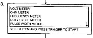
Select "VOLT METER" and press "TRIGGER".
