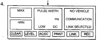
Connect test leads (RED→SIG, BLACK→COM). Measure the No.1 INJECTOR (RED→Y/B, BLACK→BATTERY negative).
