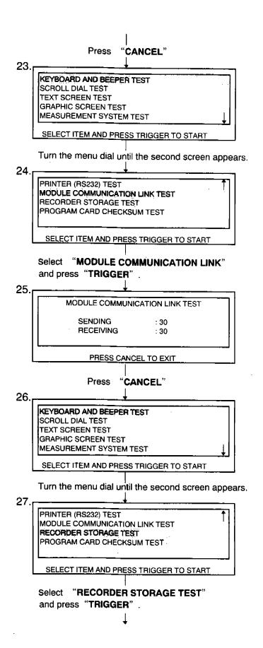
The MODULE COMMUNICATION LINK TEST checks the communication link condition.
