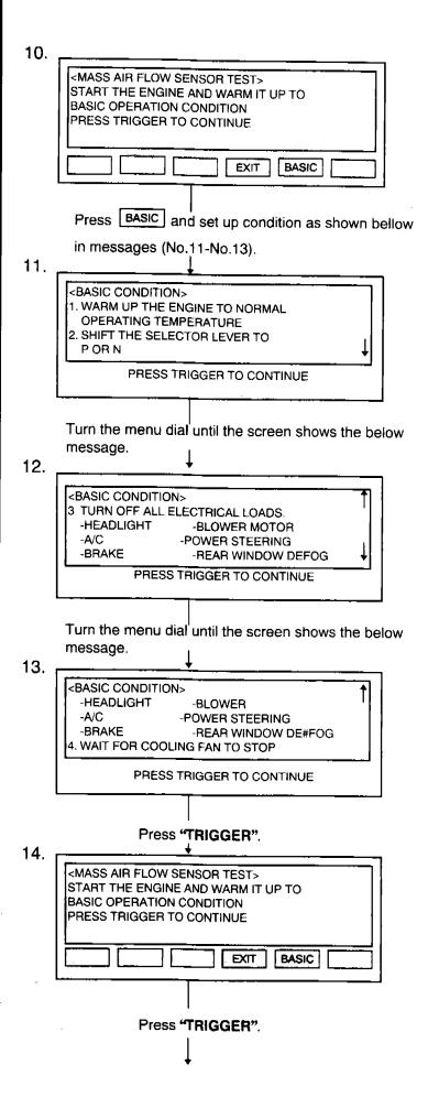
Before you carry out MASS AIR FLOW SENSOR TEST, you must set up the basic condition on your test vehicle in order to get exact test data.
