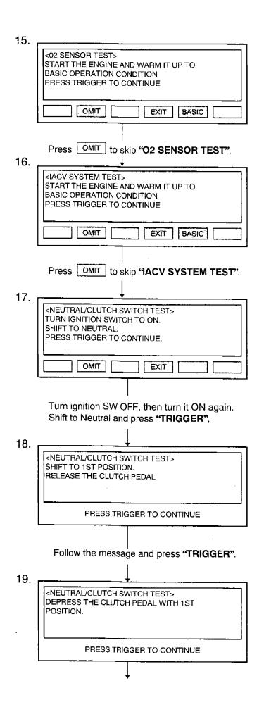
If you carry out **IACV SYSTEM TEST**, you can check the Idle Air Control Valve operation condition.
