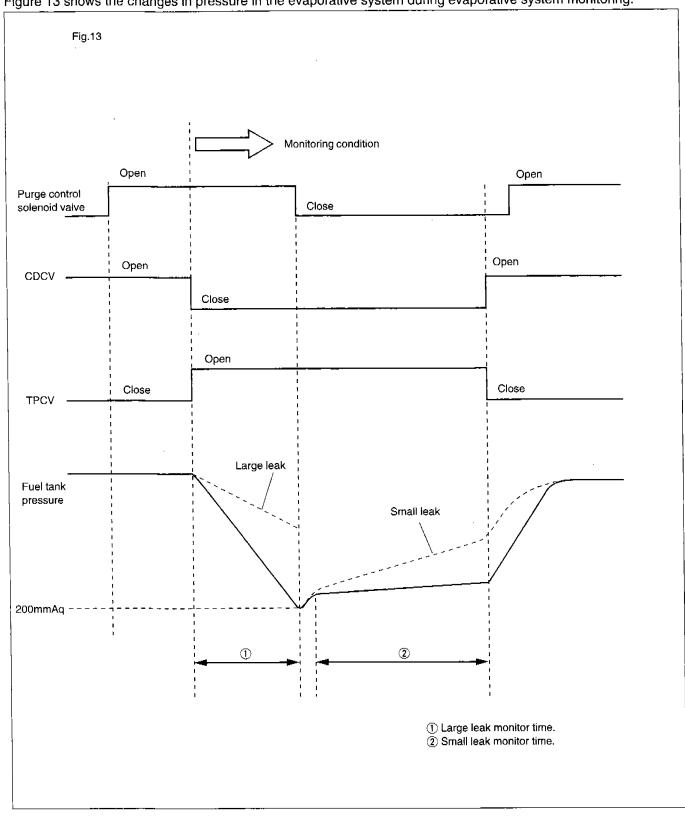
Figure 13 shows the changes in pressure in the evaporative system during evaporative system monitoring.
