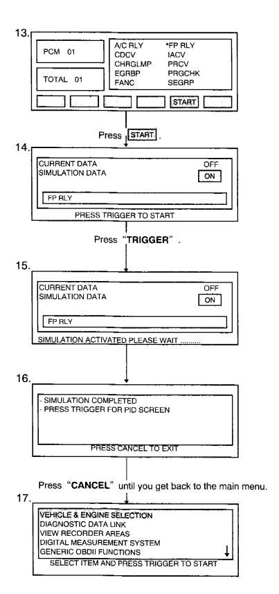
Then the fuel pump relay and the fuel pump will be operated. You can hear the fuel pump operation sound while the simulation is running. This sound lets you know that the ECM, the fuel pump and their related harnesses are all normal.
