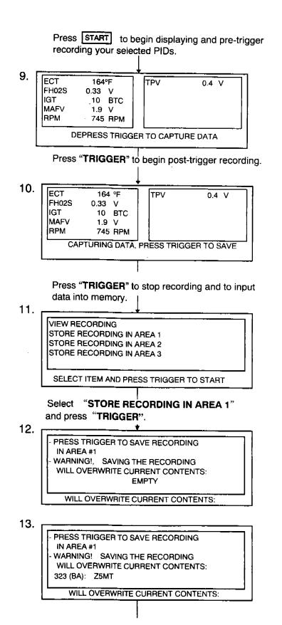
Press "TRIGGER" to save recording data in AREA 1.
