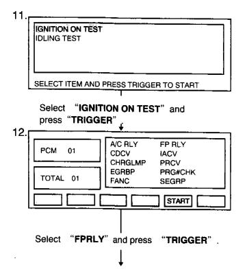
The simulation is performed for 3 seconds, and "SIMULATION ACTIVATED PLEASE WAIT" is displayed during those 3 seconds. Then INJ#1's injection will be stopped. While the simulation is performing, you can feel the idle fluctuation. This lets you know that the injector operation is normal before the testing.
