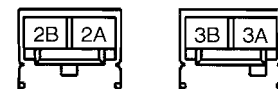
DRIVER-SIDE AIR BAG MODULE WIRING HARNESS-SIDE CONNECTOR (CLOCK SPRING ) (INFLATOR NO.1) (INFLATOR NO.2)
