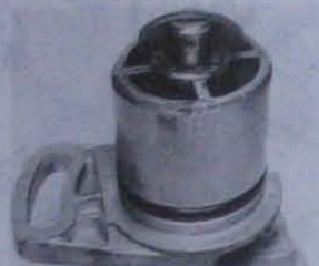
7.8 Distributor shaft drive key and roll pin
