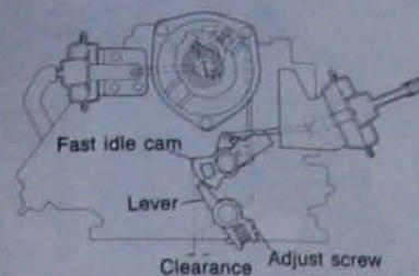
Fig. 4.14 Checking the primary throttle-to-carburettor bore clearance (fast idle cam on third step) - Aisan carburettor (Sec 12)
