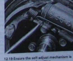
12.19 Ensure the self-adjust mechanism is in the fully retracted position (pre-September 1985 models shown).
