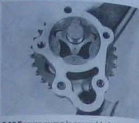
8.12 Ensure pump is assembled with rotor marks on the same side
