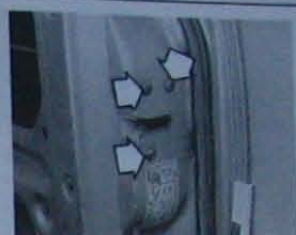
15.3 Door lock retaining screws (arrowed)
