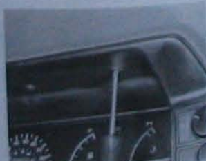
12.18A On September 1985 models onward undo the instrument panel shroud upper...
