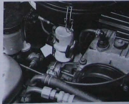
39.11 Location of the anti-afterburn valve (arrowed)
