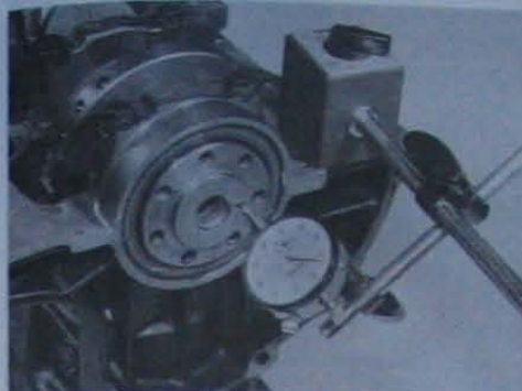
37.3 Checking the crankshaft endfloat with a dial gauge
