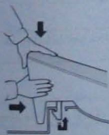
Fig. 11.12 Removing the rear seat cushion (Sec 27)
