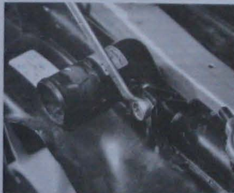
4.4A Undo the bolts securing the cooling fan cowling to the radiator...
