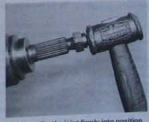
3.13B ...strike the joint firmly into position on the driveshaft
