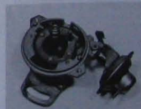
7.5 Disengage the pullrod and remove the vacuum diaphragm unit
