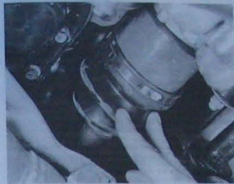
7.1 Checking the condition of the driveshaft inner constant velocity (CV) joint gaiter
