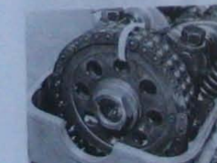
5.28 Refit the camshaft sprocket retaining nut and washer
