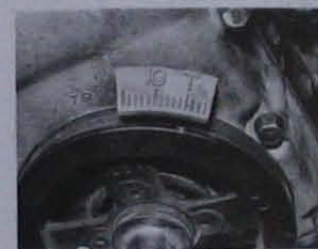
3.5 Crankshaft pulley notch aligned with TDC mark on timing scale (E series engine shown)
