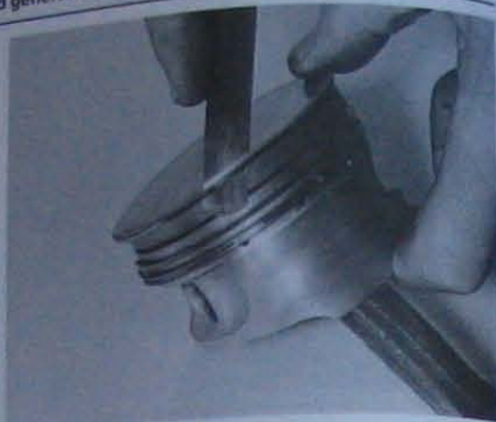
39.3 Using a feeler blade to remove the piston rings
