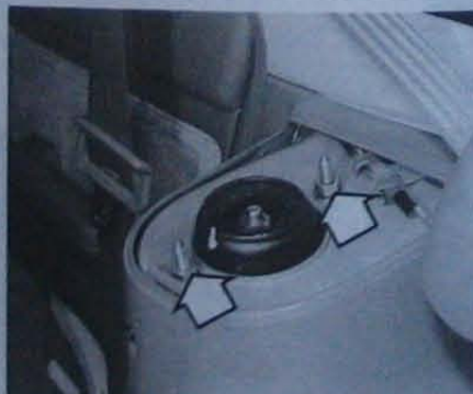
11.78 ...to gain access to the upper suspension strut mounting nuts (arrows) (Estate model shown)
