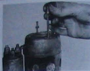
10.10 ...then install the through-bolts
