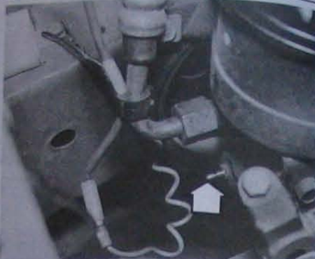
33.3 Disconnect the wire from the power steering pump pressure switch (arrowed) and connect it to earth
