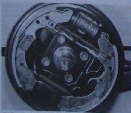
12.5 Fitted positions of shoes and springs on September 1985 models onward
