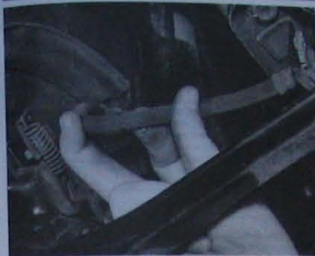
6.2 Examine the flexible hoses for signs of cracking or chafing
