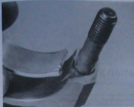
45.2 Ensure the bearing shell tab locates with the cutout in the connecting rod
