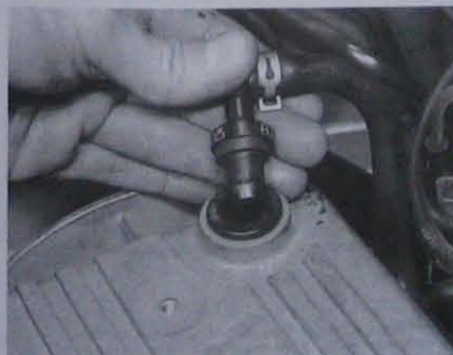
39.7 Removing the PCV valve
