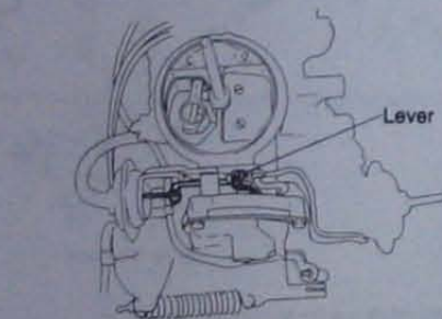
Fig. 4.13 Choke breaker diaphragm adjustment lever - Aisan carburettor (Sec 12)
