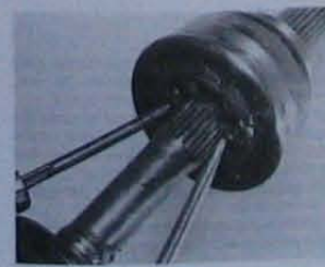
3.13A With the circlip compressed using two screwdrivers...
