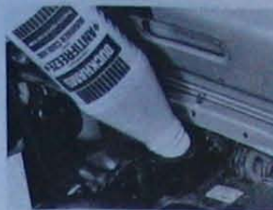
2.2 Adding antifreeze to the cooling system - early models
