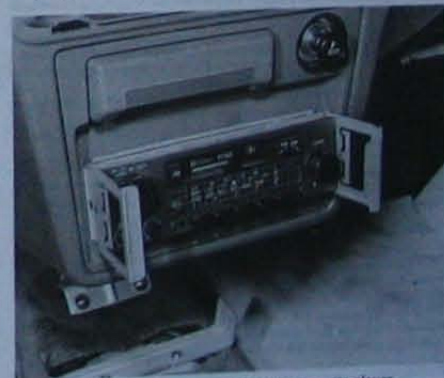
26.5 Using special tools to remove the radio cassette player September 1985 models onward
