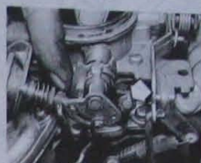
6.5 ...and disconnect the inner cable (arrowed) from the choke linkage
