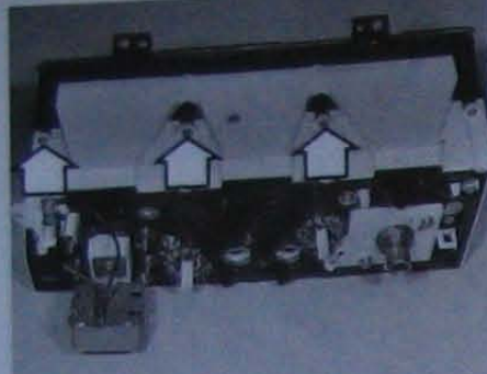
17.2 Meter cover to meter case retaining screws (arrowed) (pre-September 1985 models shown)
