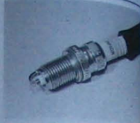
4.54 Using a short length of rubber hose to facilitate inserting the spark plugs
