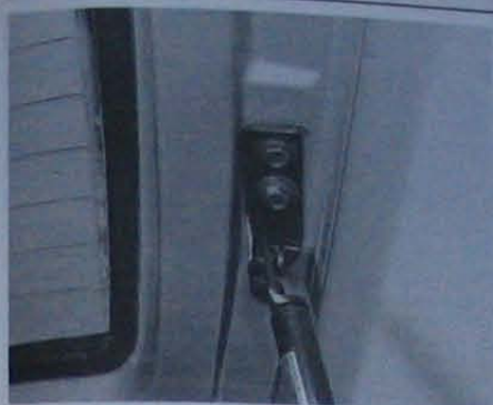
23.2A Undo the tailgate strut retaining bolts...
