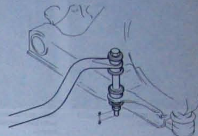
Fig. 10.9 Position the connecting link locknuts so that the specified amount of connecting link bolt thread is exposed (Sec 6)
