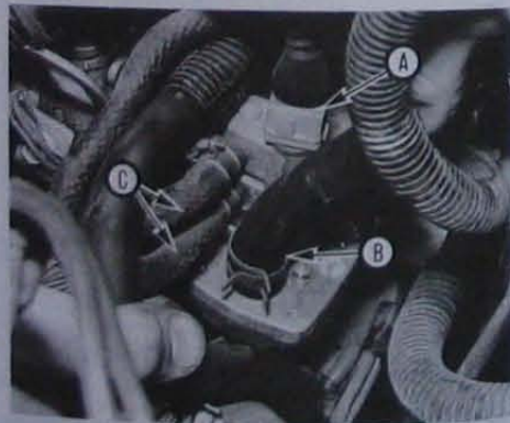
32.7 Auxiliary air valve wiring connector (A), upper hose (B) and coolant hoses (C)
