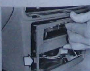
32.24B ...and prise out the side retaining tabs (arrowed) to remove lower central panel (radio removed)
