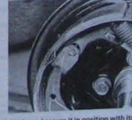
12.18 ...and secure it in position with its holding pin and spring clip (pre-September 1985 models shown)
