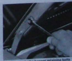
9.5 ...then undo the bonnet retaining bolts
