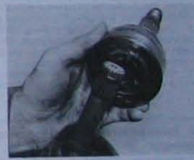
3.12 Position the joint over the splines so that it abuts the circlip
