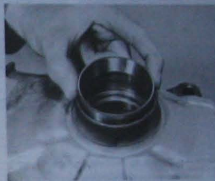
3.13 Fit the outer bearing outer race to the swivel hub
