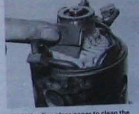
10.5 Using fine glass paper to clean the commutator
