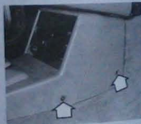
31.3A Front console section front retaining screws and sidewall retaining screws (arrowed)
