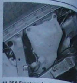
11.26A Front washer fluid reservoir location
