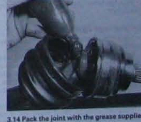
3.14 Pack the joint with the grease supplied in the repair kit
