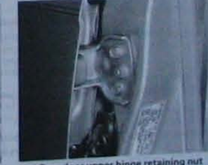
16.4 Rear door upper hinge retaining nut and bolts
