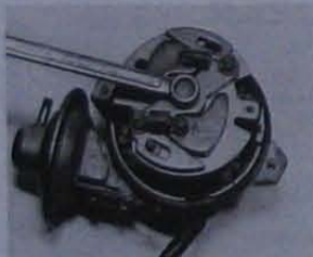
7.3A Undo the retaining bolt...
