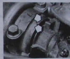
3.6 Reference marks (arrowed) made on distributor body and cylinder head
