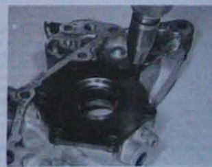
24.4 Removing the oil pump cover retaining screws
