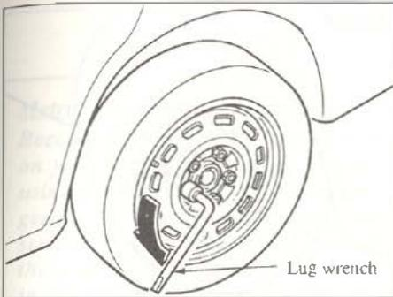
7. Loosen the lug nuts by turning them counterclockwise one turn each, but don't remove any until the tire has been raised off the ground.
