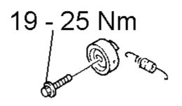
Check the tensioner and idler pulleys, renew if necessary Check the free length of the spring
