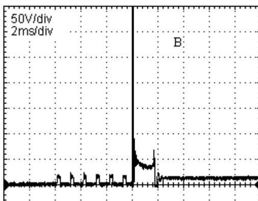
The ignition module in oscilloscope image B switches the current on and off to limit the current.
