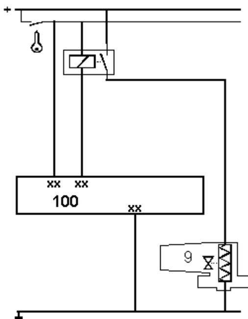
The auxiliary air valve has a connector with two terminals. One of those terminals is continuously connected with ground. The other terminal is connected with a relay switching the power to the heating element.
