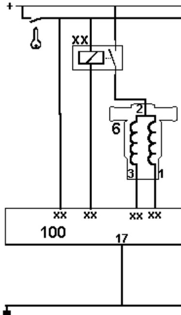
The two coils inside this type of idle speed control valve are connected with the supply voltage using one common terminal. The other two terminals lead directly to the control unit. The control unit switches the current through the solenoid on and off alternately with a duty cycle between 35 and 85%.
