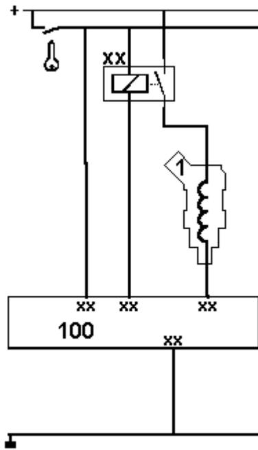
The electrical behaviour of an injector is determined by the coil inside. As a current flows through the coil the injector needle is pulled up against the spring force which causes the fuel to be injected. Two types of injector coils are used. The resistance of a normal coil is approximate 15 ohms. Other injection systems use low resistance coils (approximate 1-2,5 ohms).
