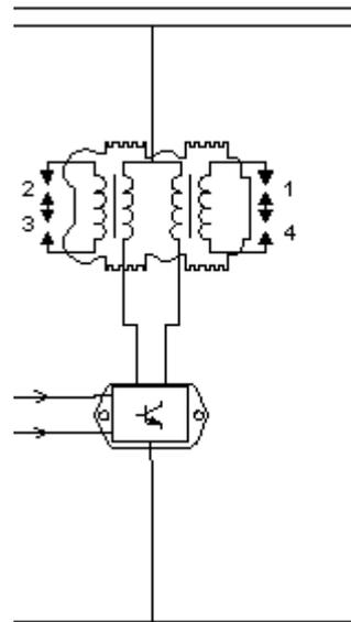
a wasted spark ignition coil on a 4- cylinder 4-stroke engine
