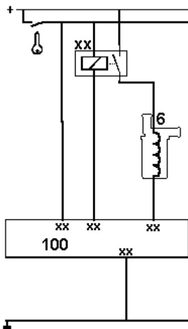
As a current flows through the coil the armature is turned against the spring force. As the current increases the airflow and the idle speed increases. If the current through the coil is switched off due to a malfunctioning system, the valve is forced into a position which results in a (too) high idle speed.
