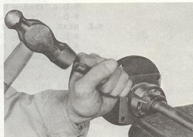
Fig. 9-4 Cutting bearing retaining collar
