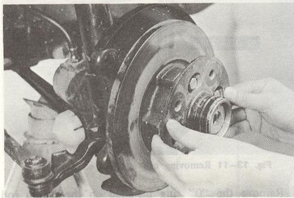
Fig. 13-3 Removing hub and rotor assembly
