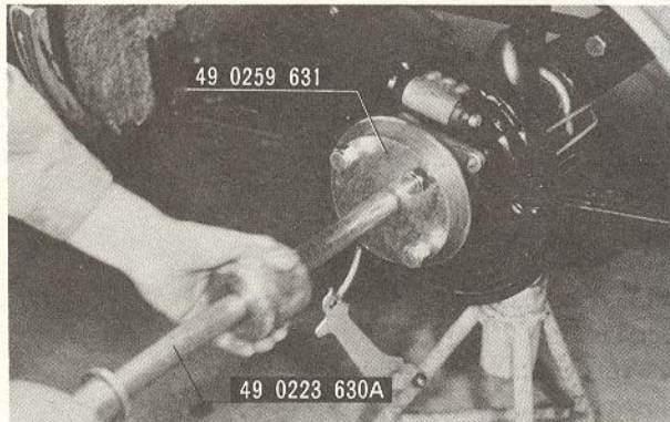
Fig. 9-1 Removing rear axle shaft
