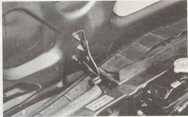
Fig. 14-2 Removing hinge attaching bolts
