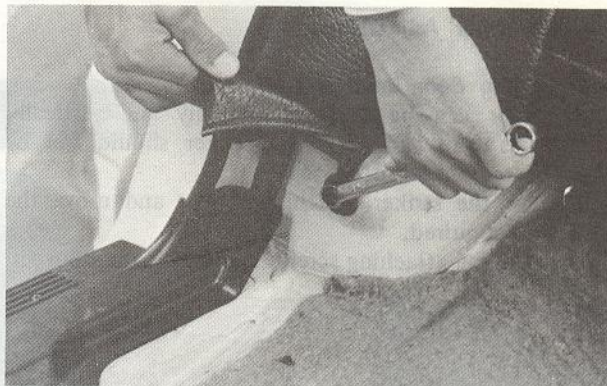
Fig. 14-44 Removing attaching bolts
