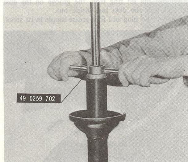
Fig. 13-39 Tightening cap nut temporarily
