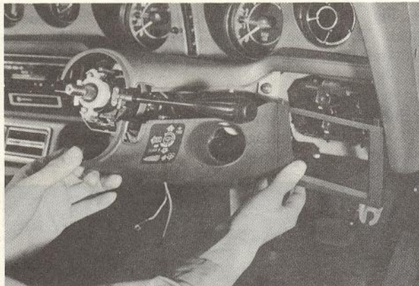
Fig. 15-25 Removing column cover
