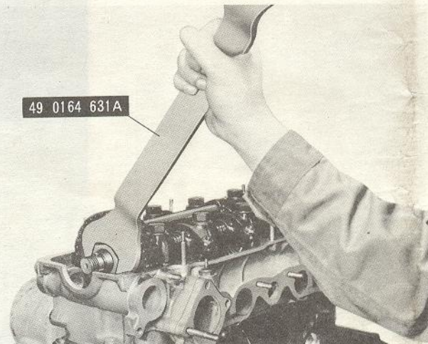
Fig. 1-5 Loosening camshaft sprocket locknut
