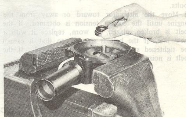
Fig. 3-22 Installing seal assembly
