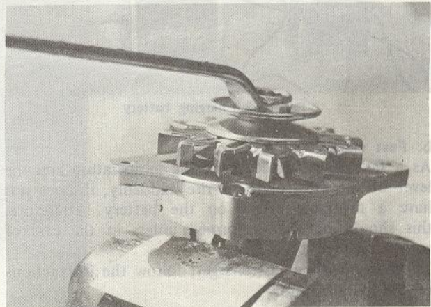
Fig. 5-7 Loosening pulley nut
