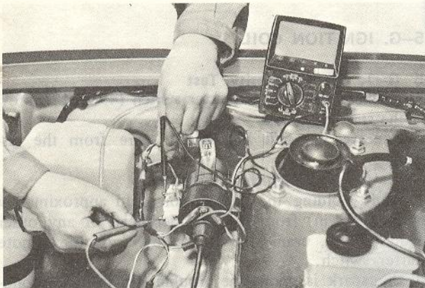
Fig. 5-63 Checking resistance of resistor
