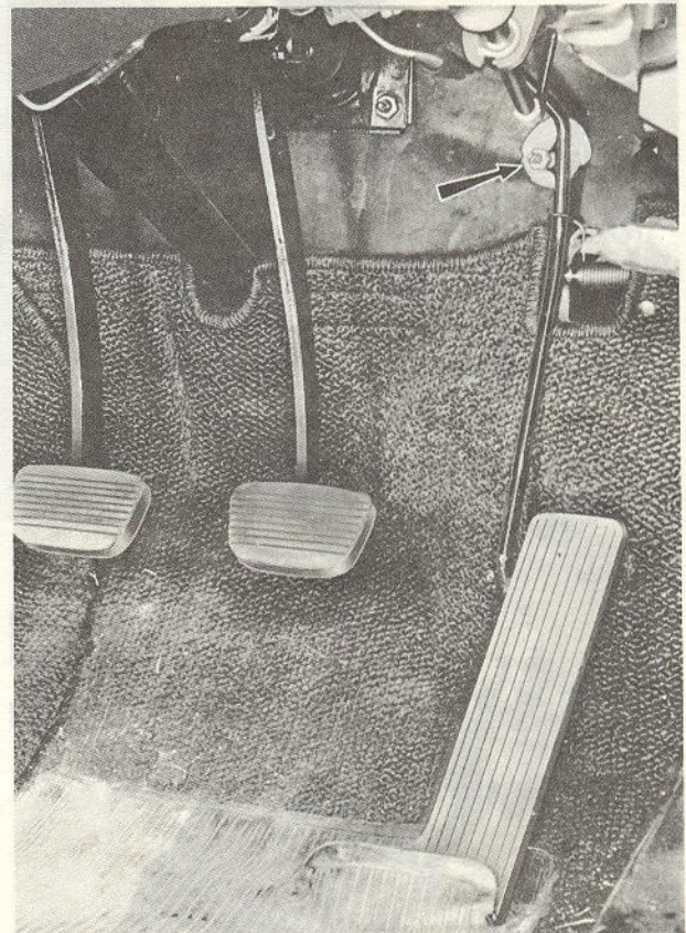
Fig. 4-12 Pedal angle adjusting screw
