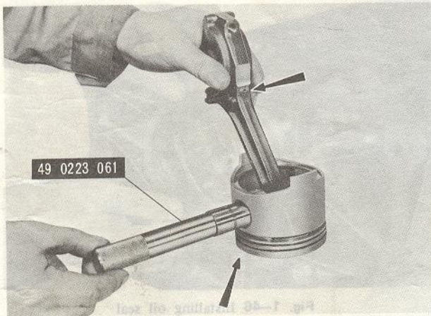
Fig. 1-38 Installing piston pin
