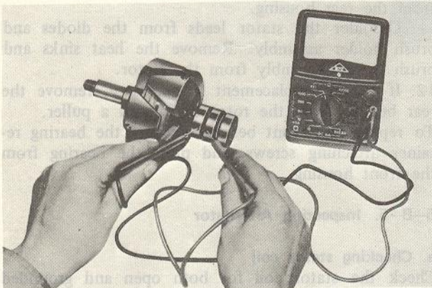
Fig. 5-14 Checking rotor for open
