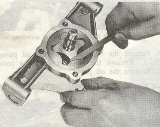
Fig. 2-8 Checking clearance between rotors
