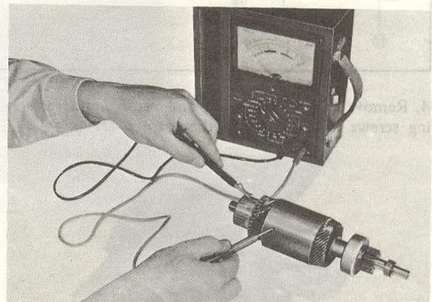
Fig. 5-32 Checking armature for ground
