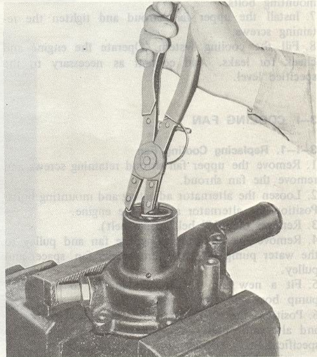
Fig. 3-21 Installing snap ring
