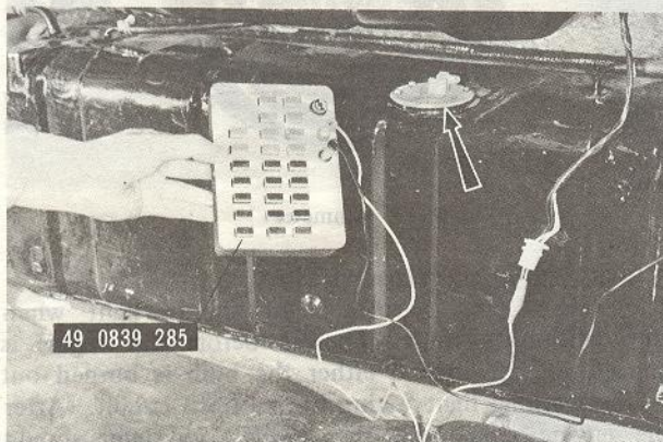
Fig. 5-66 Checking fuel gauge
