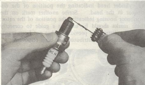
Fig. 5-43 Checking spark plug gap
