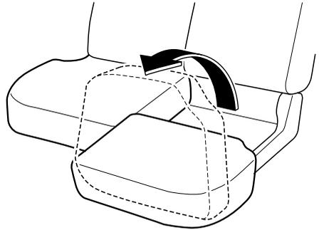
5. Pull the lock release up and fold each seatback forward.
