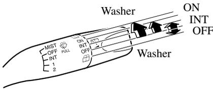
Turn the wiper on by turning the knob.
