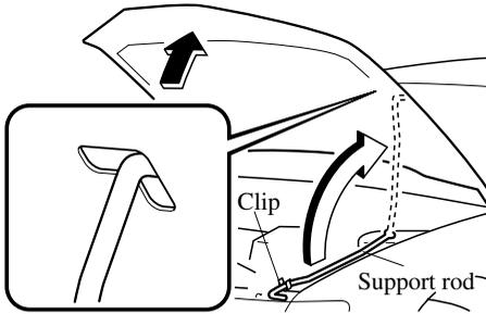
Before closing the hood, secure the rod in its clip.
