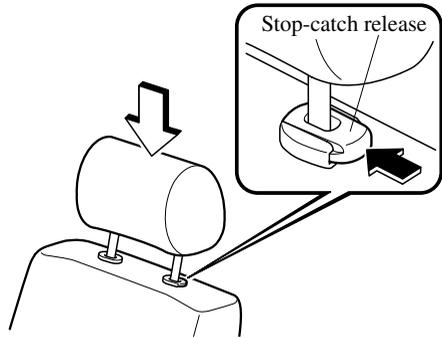
Adjust the head restraint so that the top parallels the top of the passenger's ears, never the passenger's neck.
