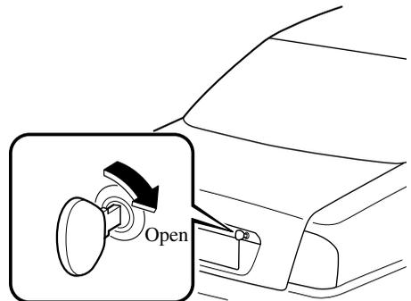
To close, use both hands to push the lid down until the lock snaps shut. Don't slam it. Then pull up on it to make sure it's secure.
