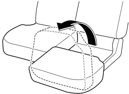
3. Pull the retaining clip to release the lever. Remove the seat bottom.
