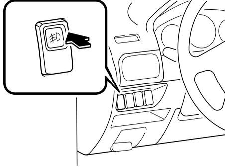
To turn on the fog lights, first turn on the headlight switch. Then press the fog light switch.
