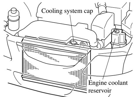
If you find no problems, the engine is cool, and no leaks are obvious, carefully add coolant as required (page 8-14).
