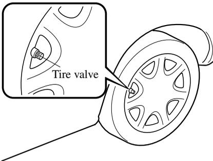
Damage could occur during installation if the wheel cover is not properly aligned.
