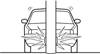
Frontal offset impact to the vehicle may not provide the stopping force necessary for air bag deployment.
