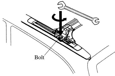
3. Tighten the bolt at both ends of the rear cross bar alternately and evenly.
