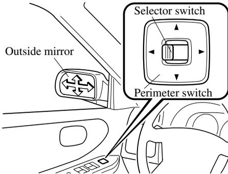
After adjusting the mirror, lock the control by moving the selector switch to the middle position.
