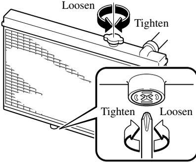
2. Only when the engine is cool, remove the radiator drain plug and drain the coolant into a suitable container.
