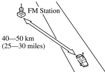
Signals from an FM transmitter are similar to beams of light because they do not bend around corners, but they do reflect. Unlike AM signals, FM signals cannot travel beyond the horizon.
