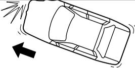
Rear-ending or running under a truck's tail gate may not provide the stopping force necessary for air bag deployment.
