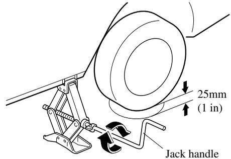
6. Remove the lug nuts by turning them counterclockwise; then remove the wheel.
