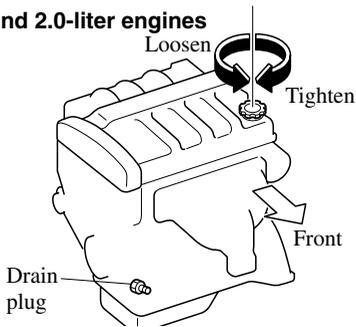
1. Warm up the engine for a few minutes and turn it off. Remove the oil-filler cap.
