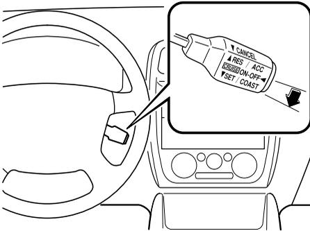
Your vehicle has a tap-down feature that allows you to decrease your current speed in decrements of 1.6 km/h (1 mph) by a momentary tap of the lever. Multiple taps will decrease your vehicle speed 1.6 km/h (1 mph) for each tap.
