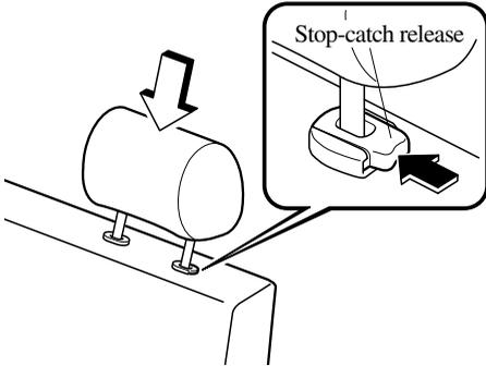
Adjust the head restraint so that the top parallels the top of the passenger's ears, never the passenger's neck.
