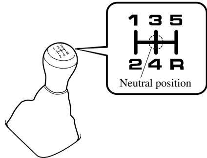
The shift pattern of the transaxle is conventional, as shown.
