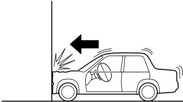
Frontal impact within about a 30 degree range from head-on to the vehicle.
