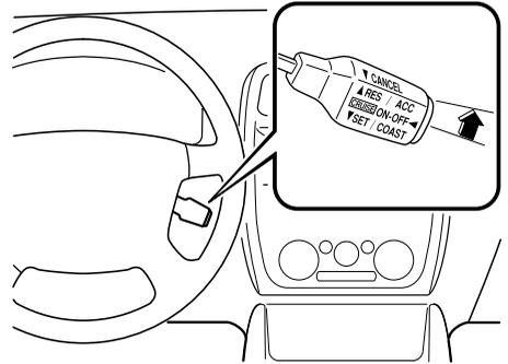
Your vehicle has a tap-up feature that allows you to increase your current speed in increments of 1.6 km/h (1 mph) by a momentary tap of the lever. Multiple taps will increase your vehicle speed 1.6 km/h (1 mph) for each tap.
