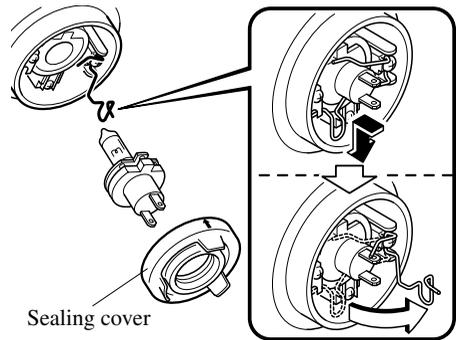
6. Swing the retaining spring out and away to free the headlight bulb.
