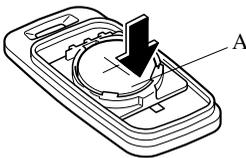
3. Install a new battery (CR2025 or the equivalent) into the front portion of the holder with the positive pole (+) facing up. Press on the B portion of the battery to set the battery.
