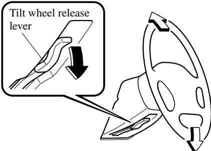
After adjusting, push the wheel up and down to be certain it's locked before driving.
