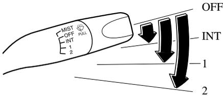
Turn the wipers on by pulling the lever down.
