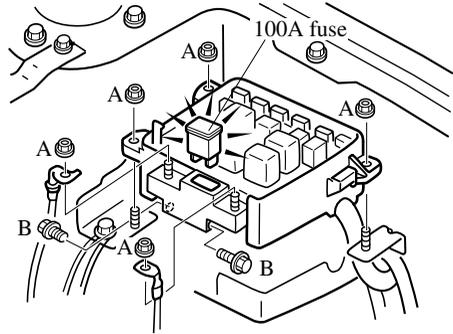
5. Replace the fuse with a new one **of the same rating**.
