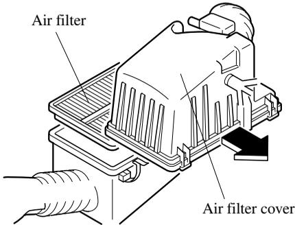
3. Wipe inside the air cleaner housing with a damp cloth.
