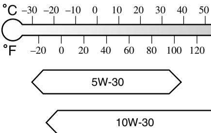
When choosing an oil, consider the temperature range your vehicle will operate in before the next oil change. Then select the recommended viscosity from this chart.
