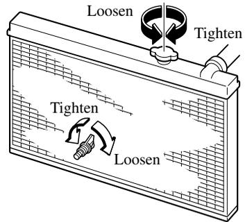
2. Only when the engine is cool, loosen the radiator drain plug and drain the coolant into a suitable container.
