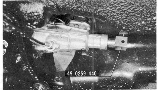
Fig. 8-2 Installing main shaft holder
