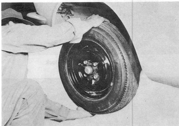
Fig. 12-20 Checking wheel bearing
