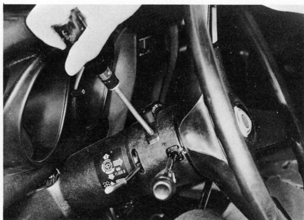
Fig. 10-23 Removing column cover
