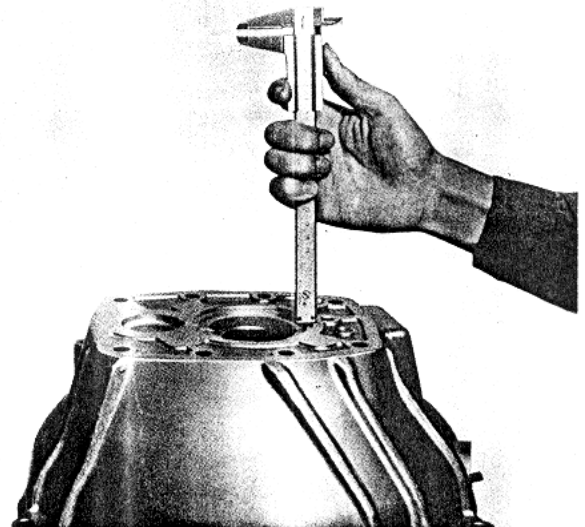
Fig. 7-38 Measuring bearing bore depth
