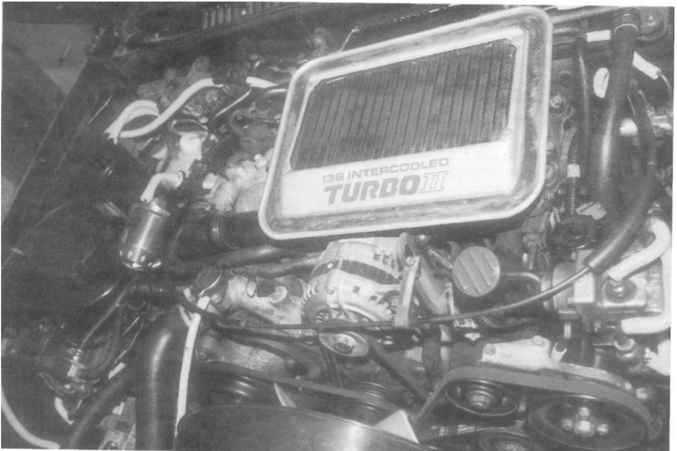
The first RX-7 to come with a factory turbo unit was the second-generation 1987 RX-7 turbo. Pictured is the intercooled "Turbo II" engine that, by 1992, was producing 200 horsepower.
