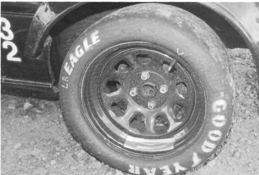
Goodyear slicks are one of the better choices for full-blown racing. Pictured here are cantilever tires that "wrap around" the rim, extending the contact surface by several inches. That way, you can use a smaller wheel (often specified by SCCA for "prepared" classes) but still get the benefit of a much wider wheel.
