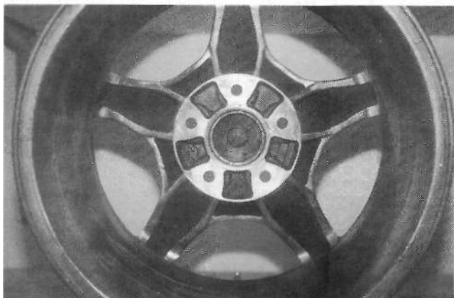
The two wheels pictured were both Mazda OEM alloys for 1993 RX-7s. Viewing the back of each wheel reveals that the one on the right seems slightly more reinforced. Mazda changed wheel subcontractors halfway through the 1993 production year, since the lighter rims had a tendency to crack. The stronger wheel weighs 1.5 pounds more than the earlier wheel. Dale Black
