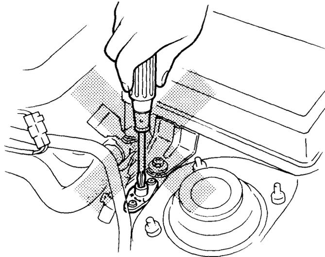
Throttle sensor adjustment: Not usually necessary unless throttle sensor unit is replaced. Throttle-idle-position auto-adjusting system automatically compensates.
