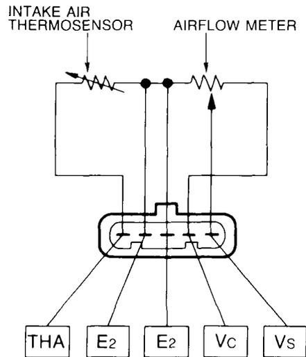
The air flow meter is changed from a vane type to a linear type. The sliding core moves parallel to the air flow. In this design, there is little air damping and low air resistance as a result of the streamlined shape.
