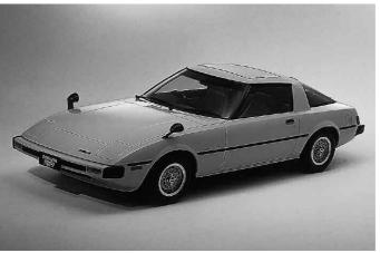
The first generation RX-7 was launched in March 1978. The front mid-ship layout with an improved 12A engine and the then-unique retractable headlights helped realized an aerodynamic body design. This model became extremely popular not only in Japan but also in North America. A face-lift was made in 1980, the new 6PI engine was installed in 1981, and the 12A turbo rotary engine, which developed 165PS added in 1983.
